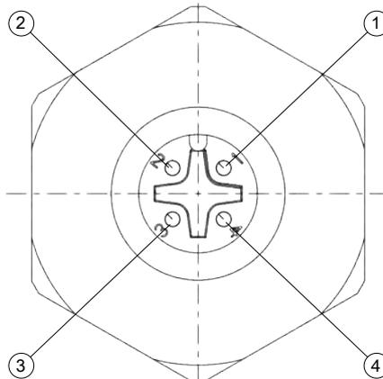
Illustration 37: Pin diagram - seen from pin side
