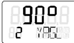
Note that the transmission ratio selector must be in the 90° position.
