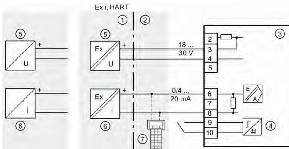
Illustration 29: 4-wire connection of 2/3/4-wire device
