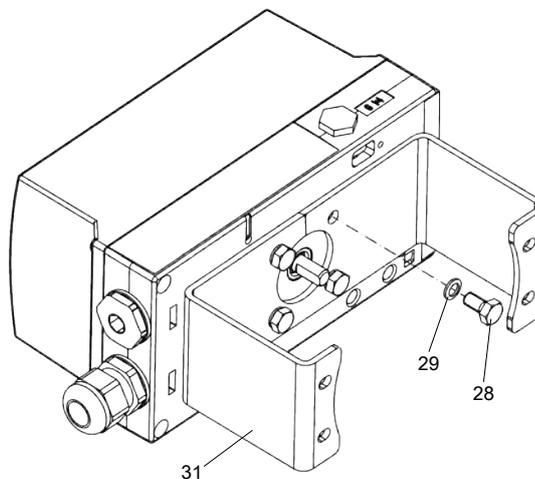
*Illustration 18:* Mounting the positioner on the bracket
