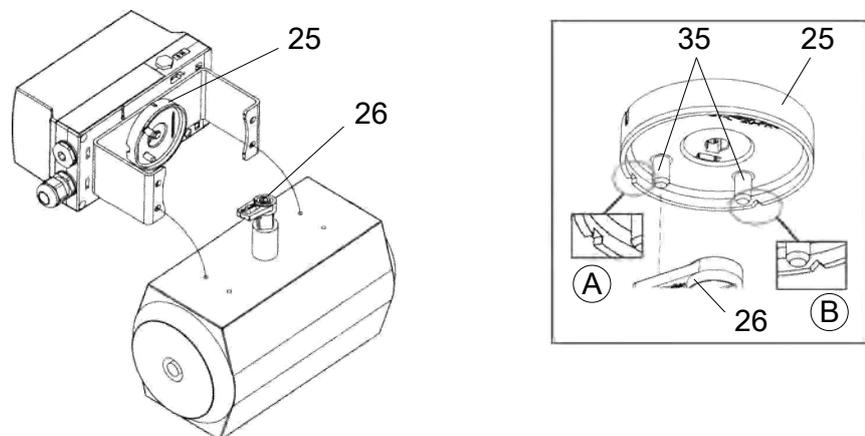
Illustration 21: Mounting the positioner on the actuator
