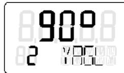
This value must absolutely correspond to the setting of the transmission ratio selector (33° or 90°).
