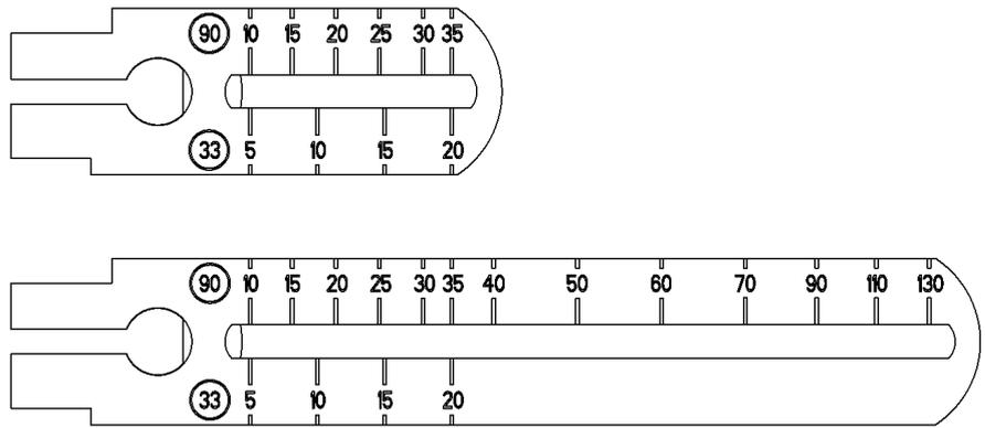
Illustration 13: NAMUR lever 3 mm to 35 mm (1), NAMUR lever > 35 mm to 130 mm (2)
