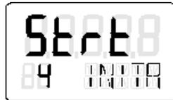
"RUN1" to "RUN5" appear in sequence in the lower display during the initialisation process. Depending on the actuator, the initialisation can take up to 15 minutes and is completed when the following display appears:
