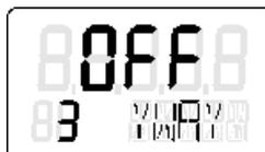
You only have to set this parameter if you want to have the total stroke determined displayed in mm at the end of the initialisation phase. To do this, you select the value in the display at which you have set the driver pin on the scale at the lever.
