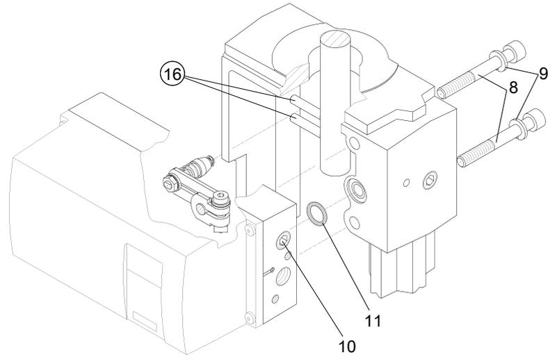
Illustration 12: Mounting the positioner on the actuator
