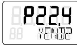
Now use the  $\triangle$  and  $\nabla$  buttons to move the actuator to the position that you wish to define as the second end position. Then press the
