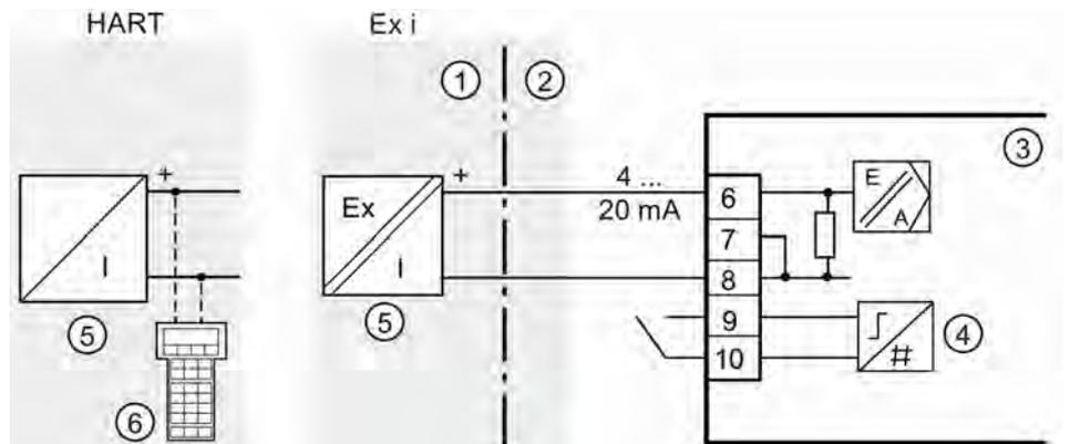
Illustration 26: 2-wire connection of 2-wire device
